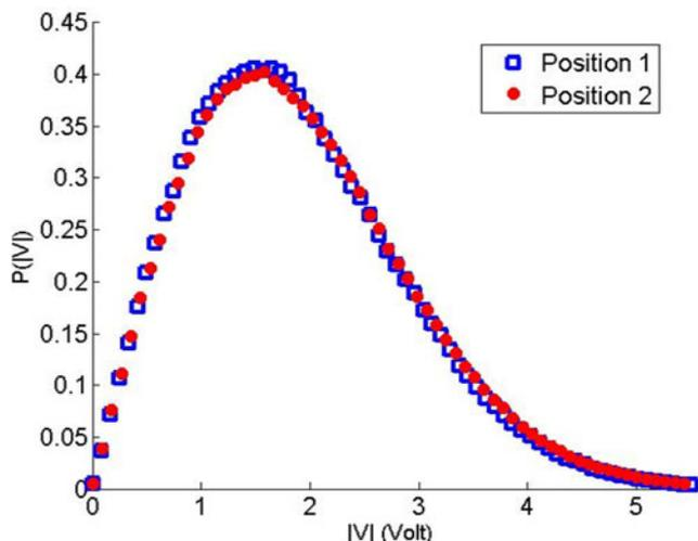
Fig. 8. Comparison of PDFs of the induced voltages on port 2 measured with the source monopole at the original location of port 1 (blue squares) and at the alternative location of port 1 (red dots) from 8.0 to 8.1 GHz.
