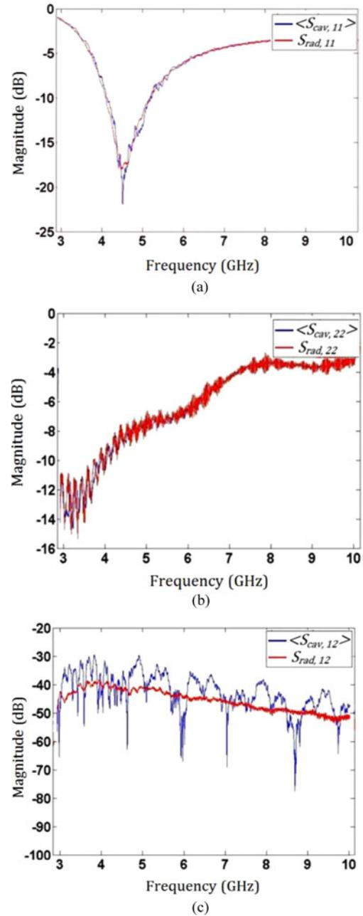
Fig. 4.  $\mathcal{S}_{\text{rad}}$  and  $\langle \mathcal{S}_{\text{cav}} \rangle$  comparisons. Fig. 4 (a), (b), and (c) shows comparisons of  $\mathcal{S}_{\text{rad}}$  and  $\langle \mathcal{S}_{\text{cav}} \rangle$  for  $S_{11}$ ,  $S_{22}$ , and  $S_{12}$ , respectively.
