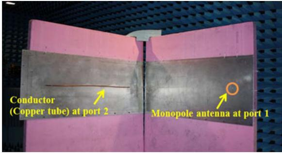
Fig. 3. Setup of free space radiation measurement.
