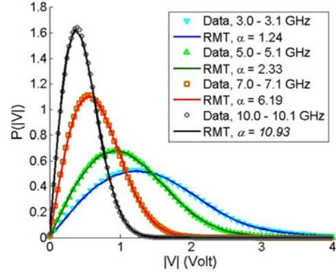
Fig. 7. Comparison of numerical RCM PDFs and experimental PDFs of the induced voltages on port 2 in frequency windows: 3.0–3.1 GHz (with  $\alpha = 1.24$ ), 5.0–5.1 GHz (with  $\alpha = 2.33$ ), 7.0–7.1 GHz (with  $\alpha = 6.19$ ), and 10.0–10.1 GHz (with  $\alpha = 10.93$ ).
