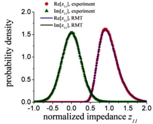
Fig. 2. PDFs of the real and imaginary parts of  $z_{11}$  generated experimentally (red circular labels and green triangular labels) and numerically (blue and black curves) for the frequency range 6.0–6.1 GHz. The distribution of the imaginary part has a zero mean and is symmetric while the distribution of the real part is not.
