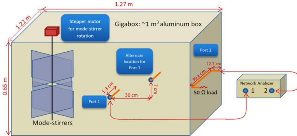
Fig. 1. Schematic diagram of the experimental setup. The GigaBox has mode-stirrers which are rotated with a LabVIEW controlled stepper motor. It has two ports that are connected to a network analyzer. The network analyzer operation is integrated with the LabVIEW control program. Port 2 is a U-shaped conductor whose other end is terminated with a 50- $\Omega$  load. There is an alternative location, on the wall of the GigaBox, to mount the transmitting port (port 1).
